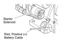
Figure 10 - Connecting Red, Positive (+) Battery Cable to Engine Starter Solenoid (Model RGH7500AIE Shown)
